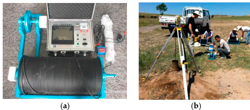
Figure 4. Borehole TV and field observation of surface borehole deformation. (a) Borehole TV; (b) Field test photo.
